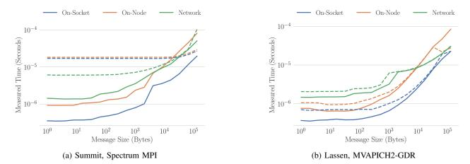
Fig. 2: The cost of communicating data directly between two CPUs (solid lines) or between two GPUs with GPUDirect (dotted lines).
