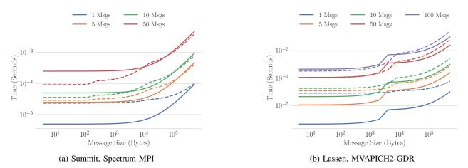
Fig. 5: The modeled cost of GPUDirect (solid) and 3-Step copy to CPU (dotted) approaches when communicating between 1 and 100 messages of various sizes.
