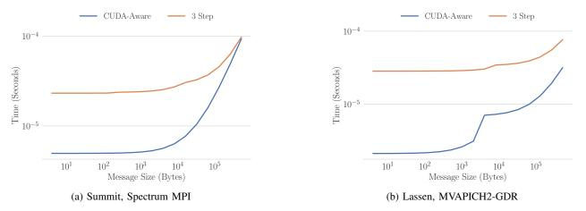
Fig. 3: The modeled cost of inter-GPU communication for various message sizes. Both viable paths of data movement are modeled, indicating that GPUDirect communication outperforms the 3-step copy to CPU method when communicating a single message between GPUs.
